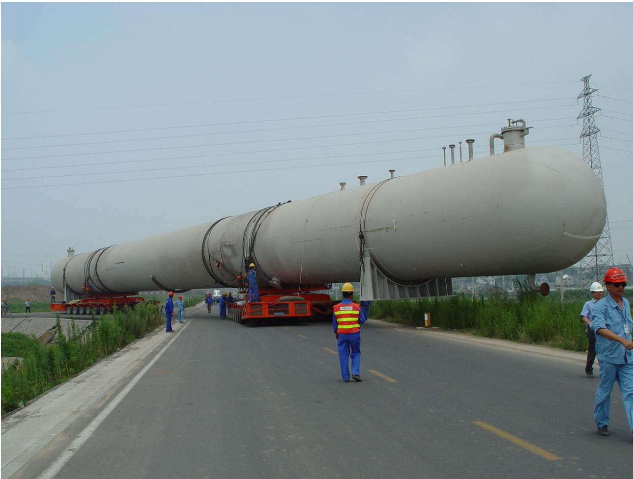
TWO 6 AXLE DOUBLE WIDE SELF PROPELLED MODULAR TRAILERS
