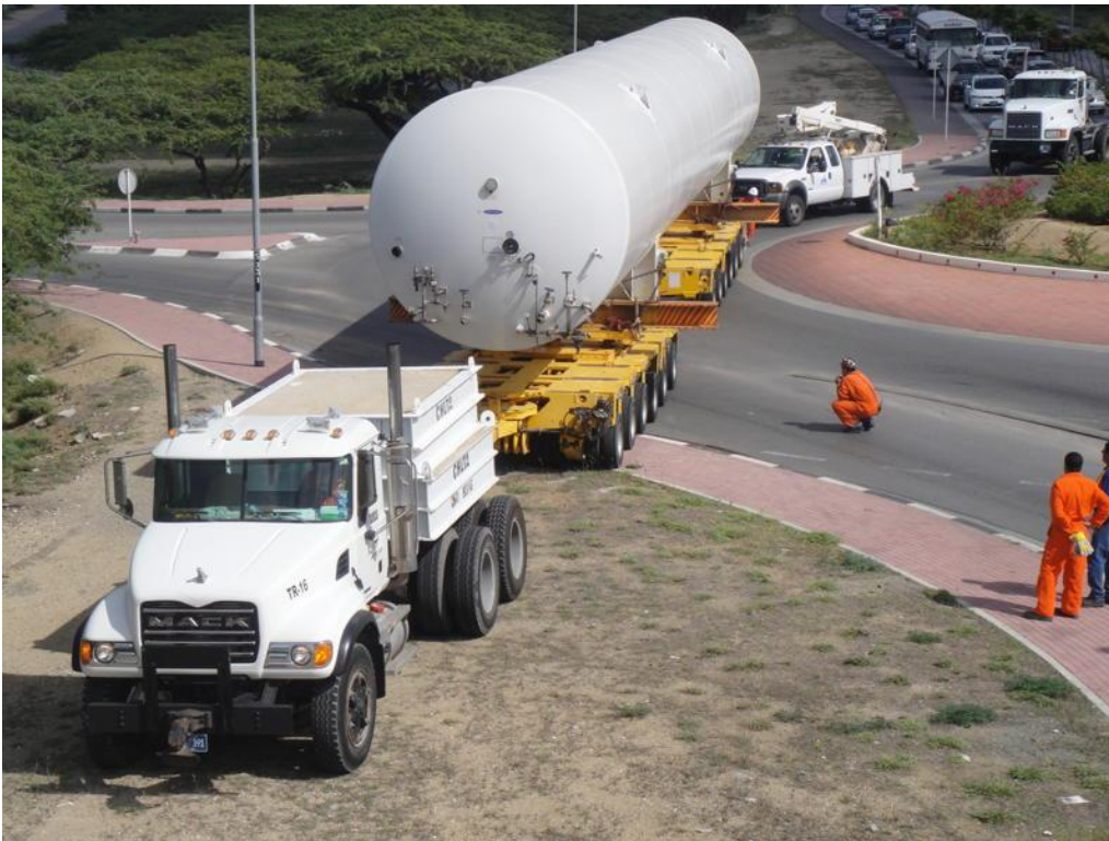
TWO, 3 METER WIDE, 6 AXLE TRAILERS HAULING A 150 Te REFINERY VESSEL
